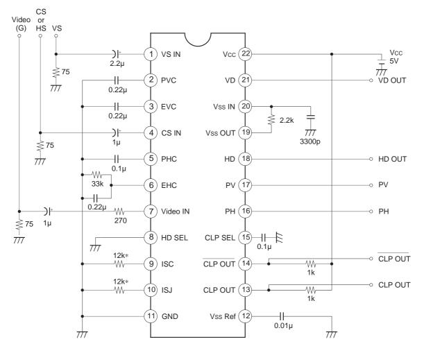
Use metal film resistor with an accuracy of  $\pm 1\%$  for the resistor marked \*.
